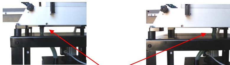
Movement of the exhaust pipe of the honing oil, inside the bench.
