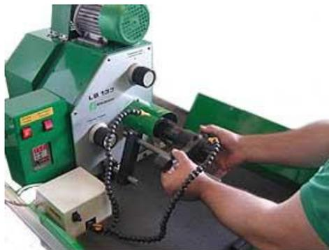
The bench honing machine is a compact unit where the piece to work is kept by hands and inserted in the hone. The material is removed by the action that the abrasive practises on the internal surface, obtained by the expansion with the longitudinal movement.
