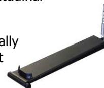
This unit have all needed characteristics to obtain a very high precision and, at the same time, includes a lubrication system that helps to quicken cut, improve the finishing, extend the abrasives life and make working much more clear and clean.
